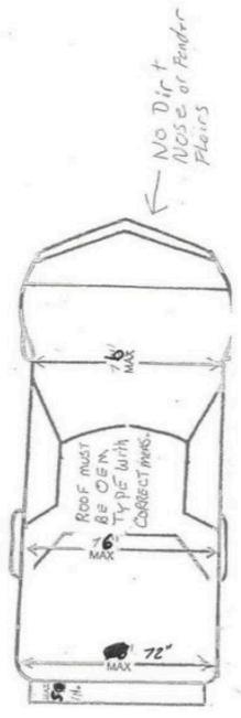
No MD3 Gen 1 or Gen 2, No Evolution 1, Evolution 2, Fivestar outlaw late model nose, Dominator Outlaw asphalt late model nose, Dominator Late model nose, Dominator D2X nose. Noses must be mounted with the lower sides parallel to the ground. Do not tilt the nose back at the top edge to gain more angle.
